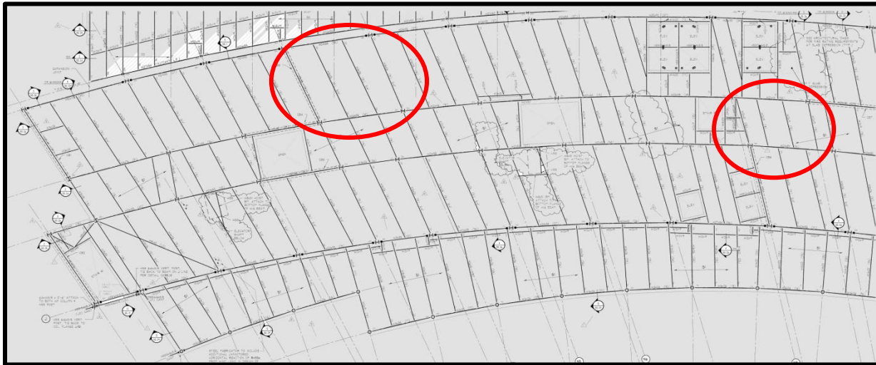
Figure 10: Typical framing plan, west wing of hospital. Typical 30'x30' bay and typical 30'x18' bay are highlighted.
