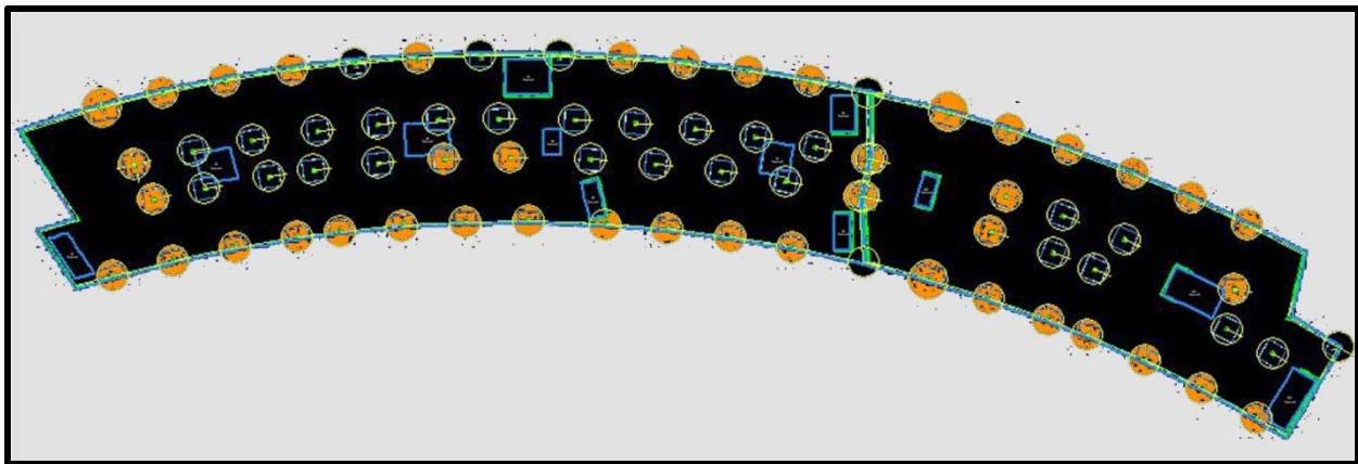
Figure 50: Design strip plan identifying locations where shear stud reinforcement was necessary to handle punching shear.
