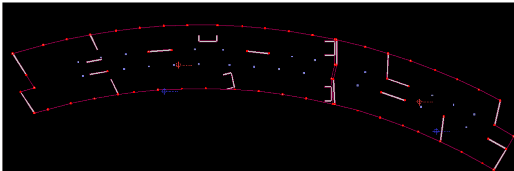
Figure 29: Trial #34 wall layout. Shear wall groups located at elevator shafts.
